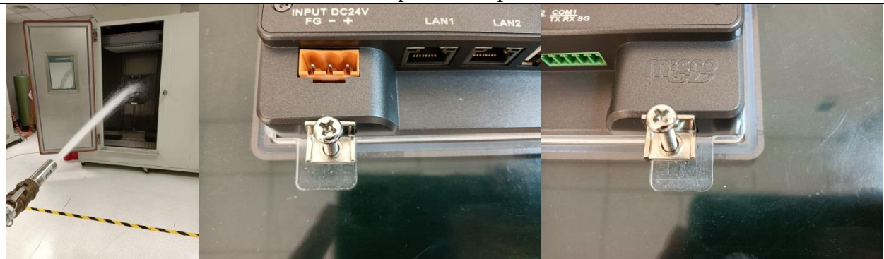
EUT internal status after waterproof test
