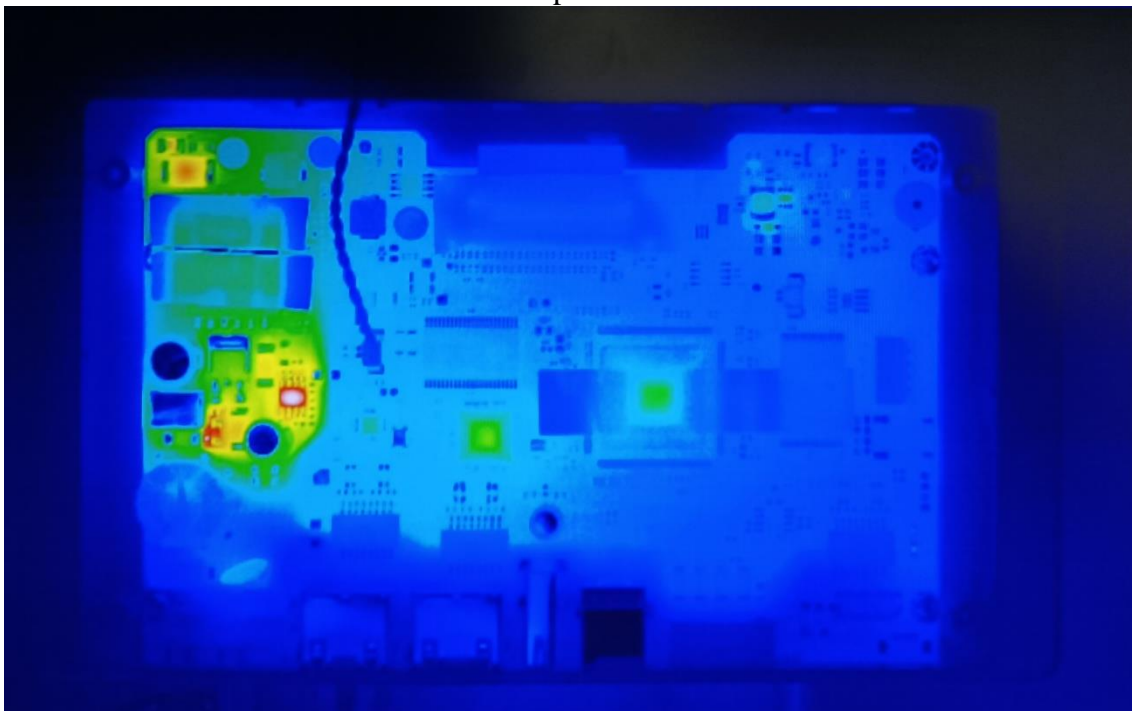
IR Picture-Reference heat distribution (Ambient 25°C)
